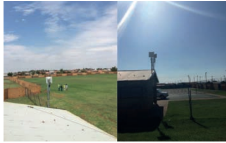
Above left: Altai's C1ns is used for pico coverage, backhaul and as CPE to extend the Wi-Fi coverage.
