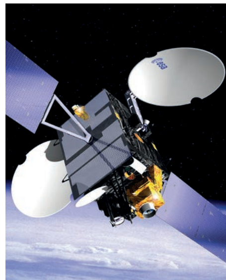
Avanti's Artemis orbits at 21.5°E and features Ka-, S- and L-band transponders.
