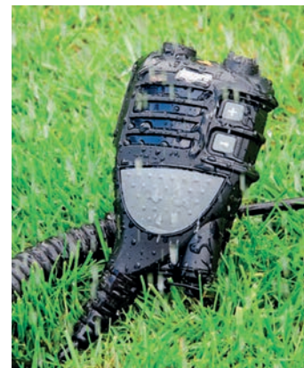
Sepura's ULTRA CSM is an IP67 rated all-weather controller speaker microphone. It can withstand 180°C and is said to be highly durable thanks to its polycarbonate casing – the same material used for riot shields.
