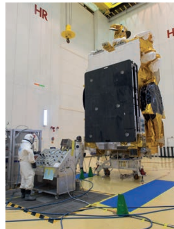
In late October, Arianespace began preparations for the launch of Arabsat-6B , seen here receiving its propellant.
