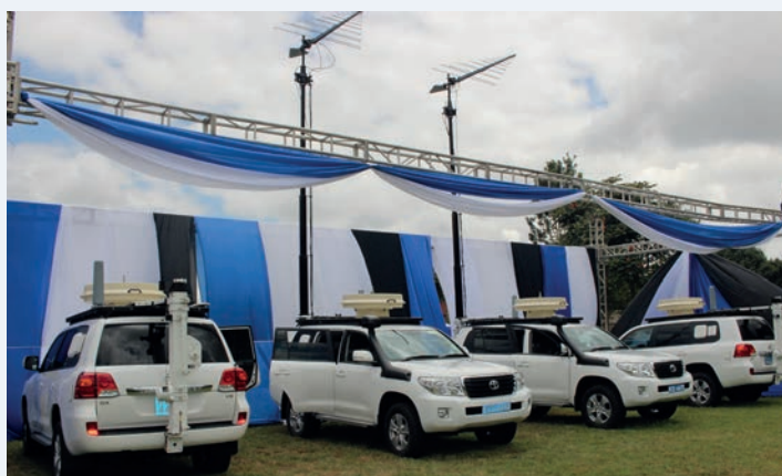
Rohde & Schwarz equipped four off-road vehicles to extend the range of the direction finding base and fix interferer positions while moving.
