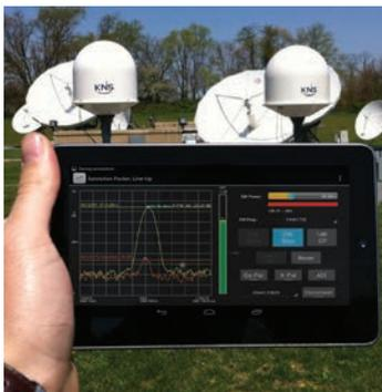
It's claimed *Satmotion* enables installers to point and adjust antennas and streamline the overall commissioning of VSAT solutions.
