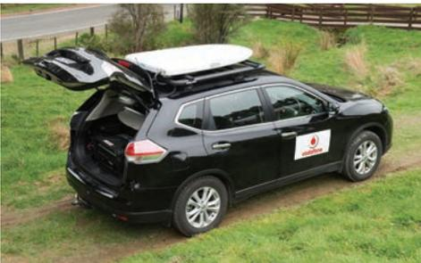
*Z-Car* is a prototype mobile network on wheels developed by Vodafone New Zealand. The vehicle has a 4G small cell built into its boot which provides coverage over a 2km radius, even as the vehicle is in motion. Download speeds of up to 10Mbps and 2Mbps upload are said to be achievable. The car can also communicate with the digital trunked radio systems used by the emergency services.
