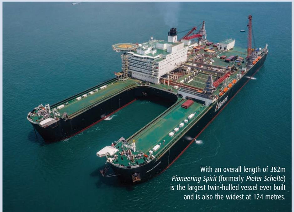
With an overall length of 382m *Pioneering Spirit* (formerly *Pieter Schelte*) is the largest twin-hulled vessel ever built and is also the widest at 124 metres.
