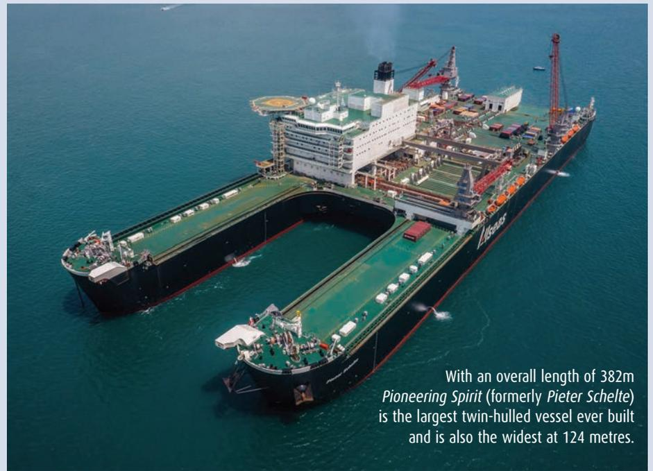
With an overall length of 382m *Pioneering Spirit* (formerly *Pieter Schelte*) is the largest twin-hulled vessel ever built and is also the widest at 124 metres.
