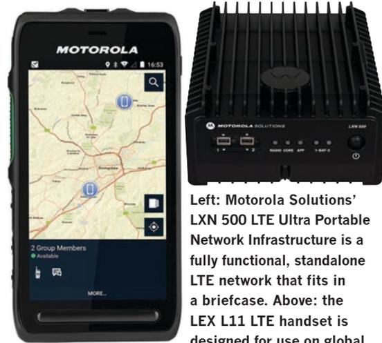
**Left: Motorola Solutions' LXN 500 LTE Ultra Portable Network Infrastructure is a fully functional, standalone LTE network that fits in a briefcase. Above: the LEX L11 LTE handset is designed for use on global broadband networks.**
