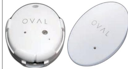
The compact OVAL sensor (left) can communicate over Wi-Fi to the gateway (right) from a distance of up to 150ft away.
