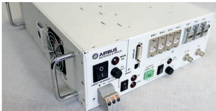
Left: Airbus Defence and Space's standalone Tactilon Cell can be used to create a small LTE network. It comprises a base station, terminals, LTE software and an app server for mission-specific apps. All the cell's features comply with 3GPP standards. Right: the recently launched Dabat integrates a complete TETRA radio and smartphone in one device. Airbus says it can work on any TETRA network.
